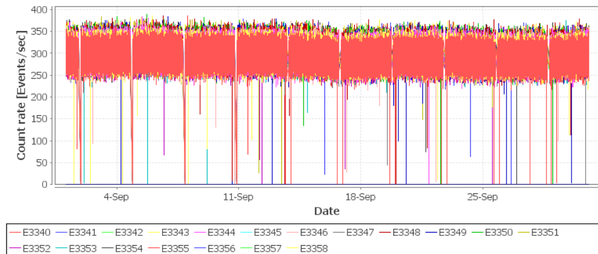
Figure 18: SPI GeD Time Tagged Saturated count rates
