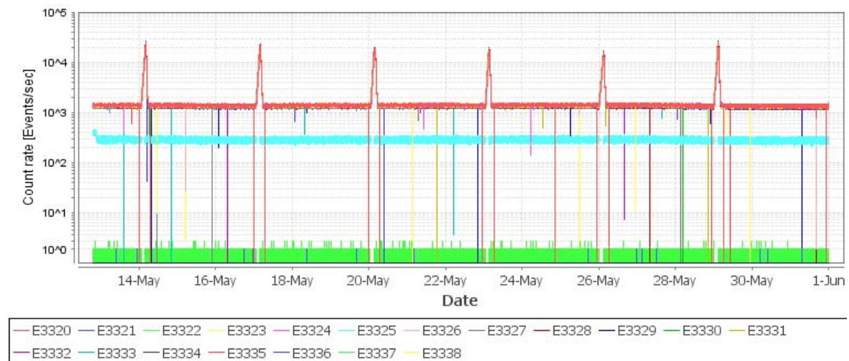
Figure 18: SPI GeD Time Tagged count rates. Note that the scale used for plotting is logarithmic
