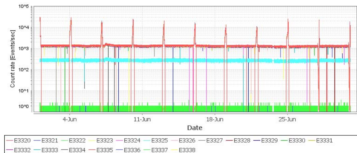
Figure 15: SPI GeD Time Tagged count rates. Note that the scale used for plotting is logarithmic
