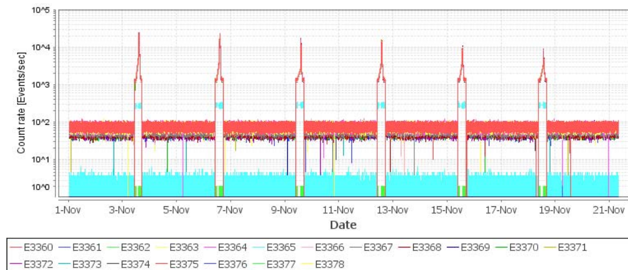
Figure 15: SPI GeD Non-Vetoed count rates. Note that the scale used for plotting is logarithmic.
