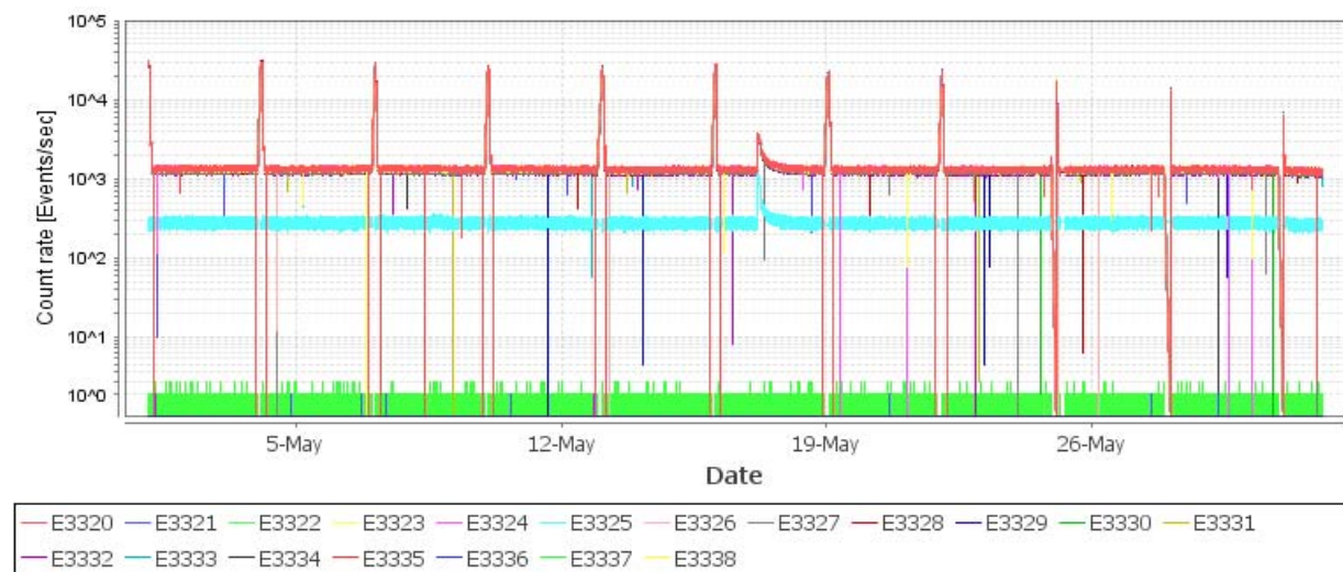
Figure 17: SPI GeD Time Tagged count rates. Note that the scale used for plotting is logarithmic.
