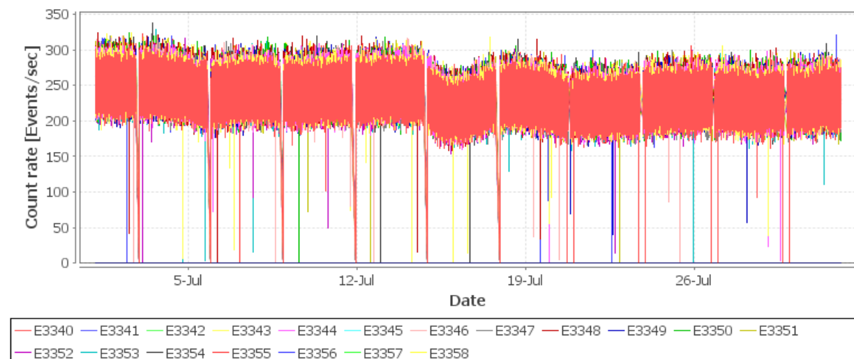
Figure 19: SPI GeD Time Tagged Saturated count rates. The impact of the increased solar radiation throughout the months can be seen.
